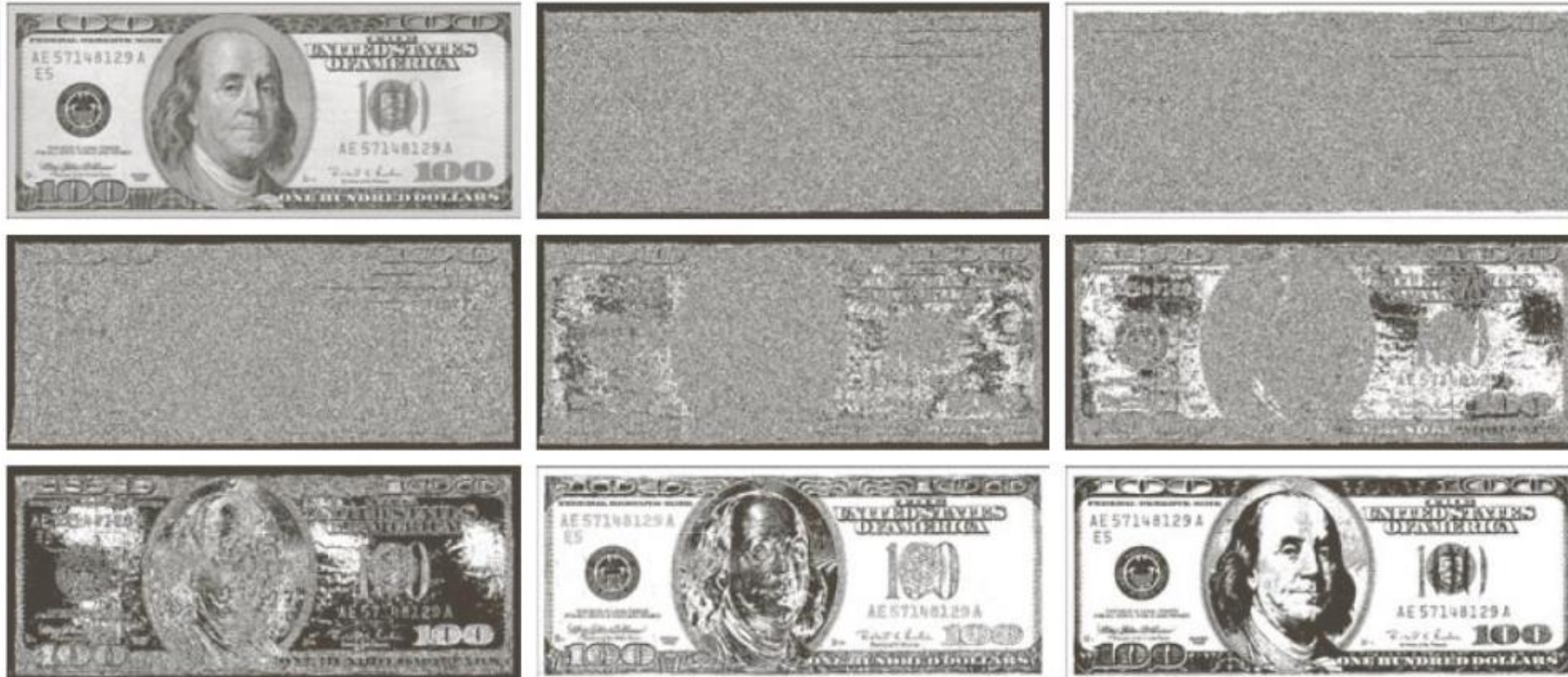
FIGURE 3.14 (a) An 8-bit gray-scale image of size 500 \times 1192 pixels. (b) through (i) Bit planes 1 through 8, with bit plane 1 corresponding to the least significant bit. Each bit plane is a binary image.
