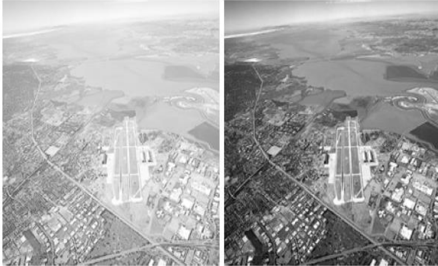
FIGURE 3.9 (a) Aerial image. (b)–(d) Results of applying the transformation in Eq. (3.2-3) with c = 1 and \gamma = 3.0, 4.0, and 5.0, respectively. (Original image for this example courtesy of NASA.)
